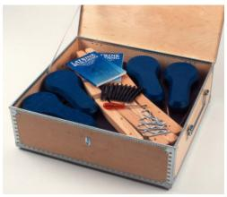
The mould box kit contains everything needed to reproduce concrete squatting plate moulds in a cost effective way. The kit is ideal for shipping so that slabs can be produced in country and therefore reduce international freight costs. Supplied in a lockable plywood box with a carry handle at each end
